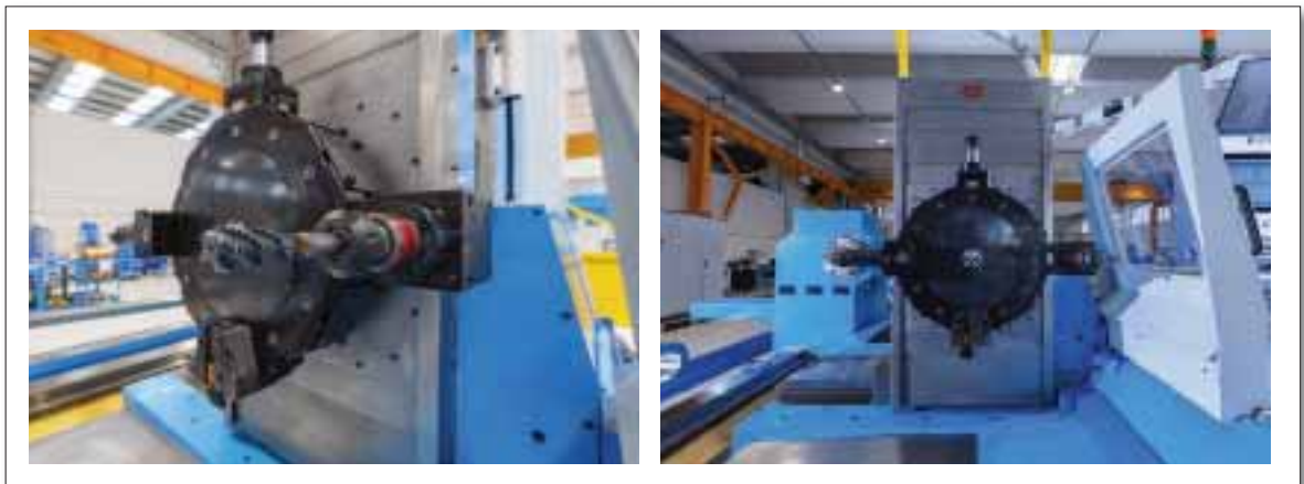
Ⓒ Fig 3 12 position heavy-duty motorized turret
