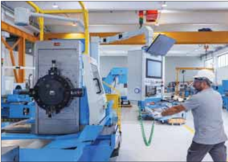
Fig 8 Overview of the latest Atomat AT925E turning a roll of 20t
