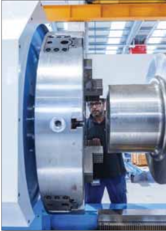
Ⓒ Fig 2 Clamping system of four independent jaws
