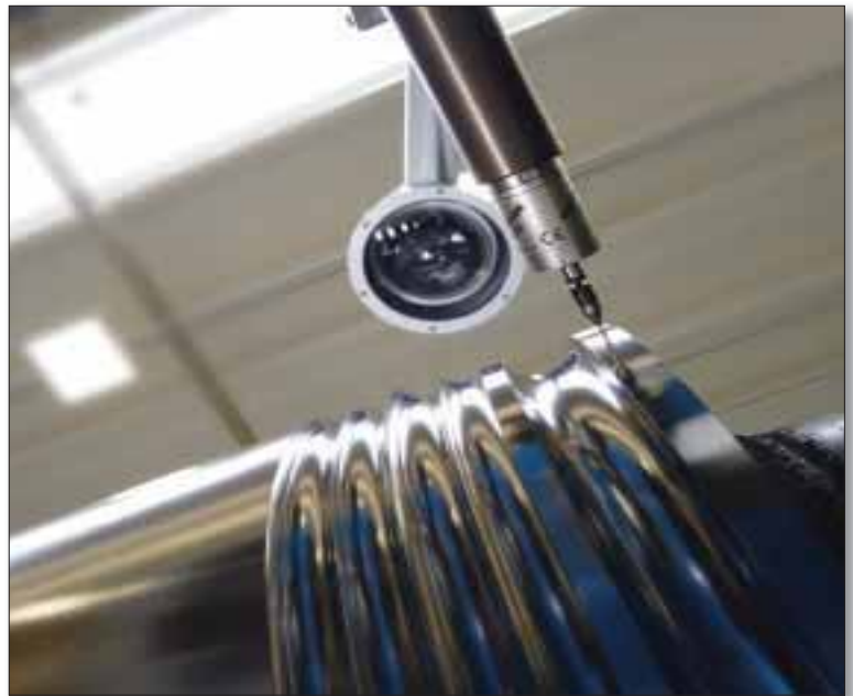
Fig 5 Probe system for in-process geometry checking
