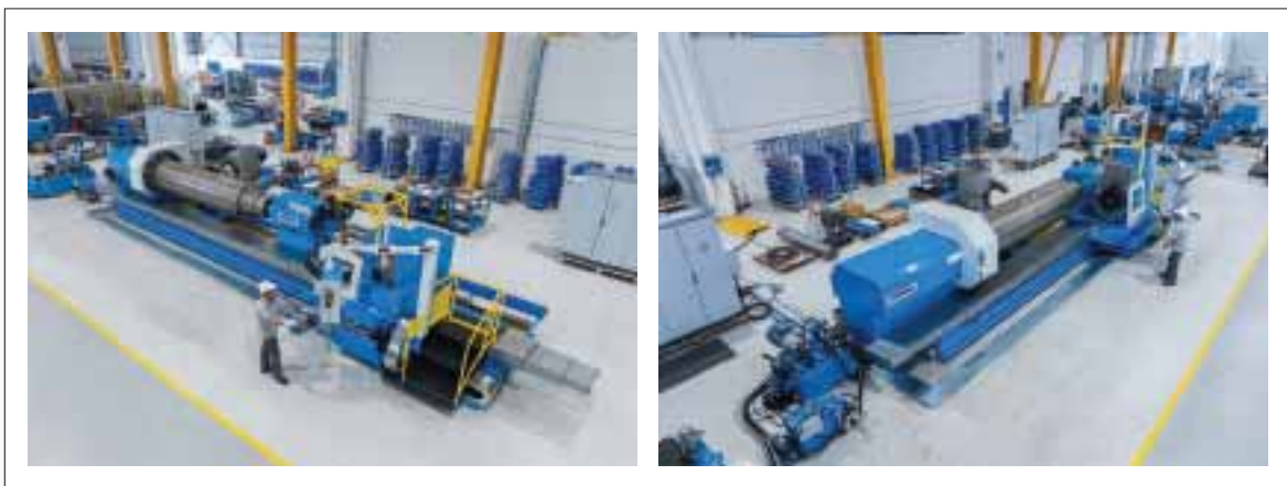
Fig 1 AT925E - Multifunctional Super-Heavy-Duty turning lathe
